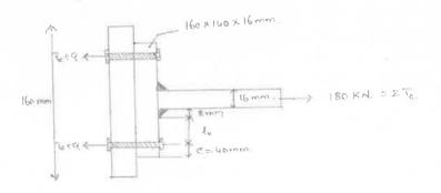
3. Calculate the size of weld for the bracket shown in figure below.
